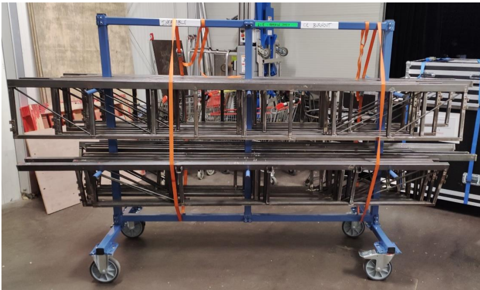
Platform trusses stored on 2 carts
